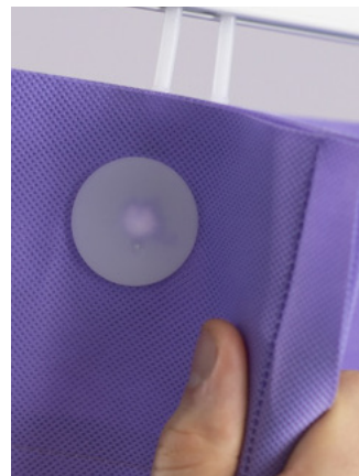
Robust hooks are ultrasonically welded.
